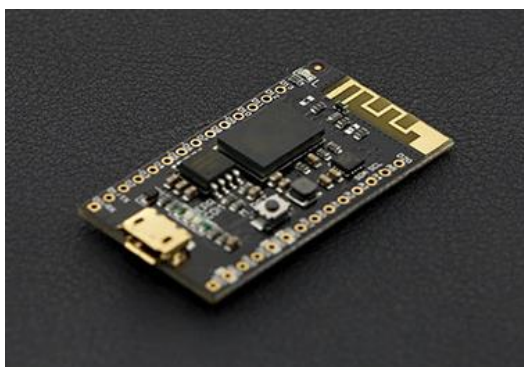
Rys. 4.2. Intel Curie Quark ARC (Dfrobot, 2019)
