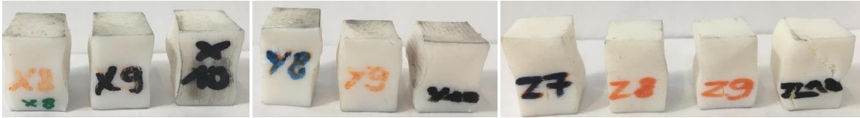
Fig. 5.15. Samples loaded in X, Y, and Z orientation after compression a strain rate 0.1 \text{ s}^{-1} (own source)
