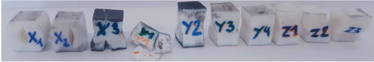
Fig. 5.13. Samples loaded in X, Y, and Z orientation after compression a strain rate 0.01 \text{ s}^{-1} (own source)
