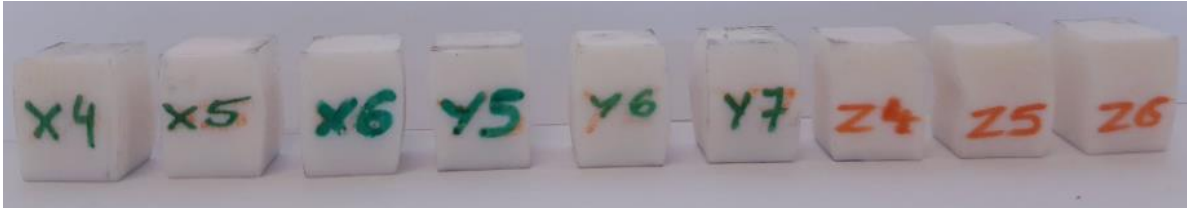
Fig. 5.11. Samples loaded in X, Y, and Z orientation after compression a strain rate 0.001 \text{ s}^{-1} (own source)
